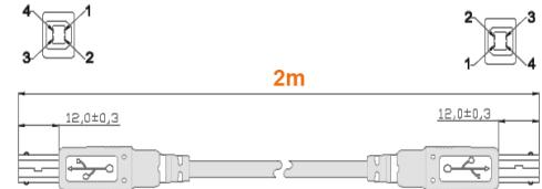
**USB 2.0 B** AWM STYLE 2725 80°C 30V VW-1 28AWG/1P 24AWG/2C **USB 2.0 B**
